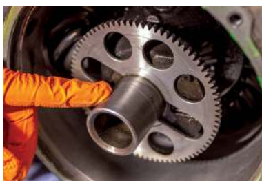
Left The outgoing bearing certainly left its mark!
