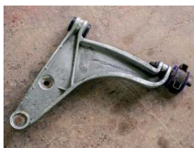
Left Every factory rubber bush is to be replaced with a Powerflex purple polyurethane part
