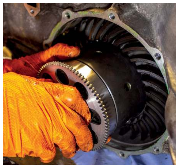
Left and below Crown wheel bolts need to be correctly torqued and thread-locked before the new differential is fitted
