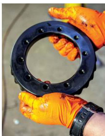
Left The crown wheel is removed from the old diff and fitted to the new Quaife ATB
