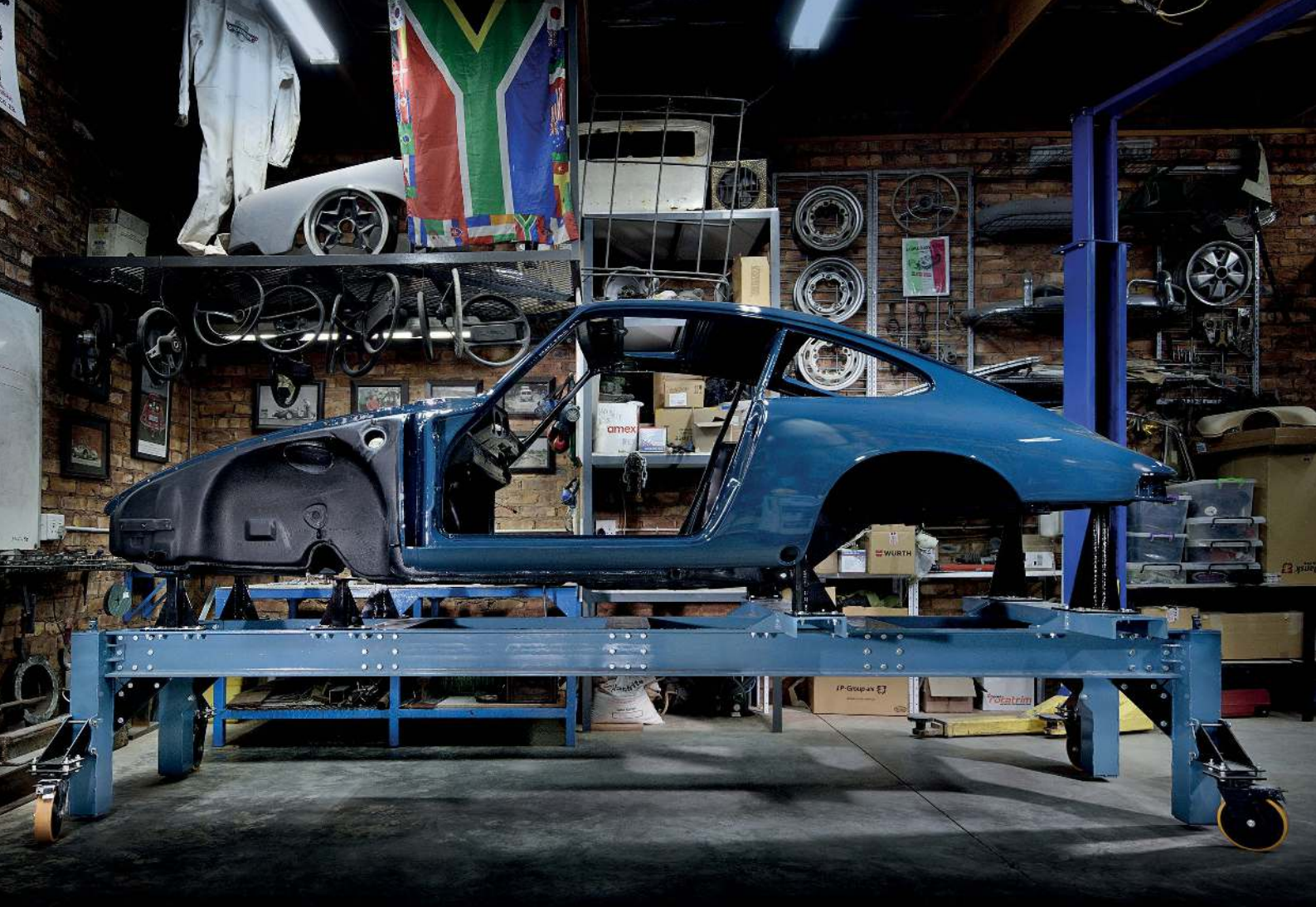
Above Structural damage required a custom jig to straighten the car before Wernher could begin with restoration work
