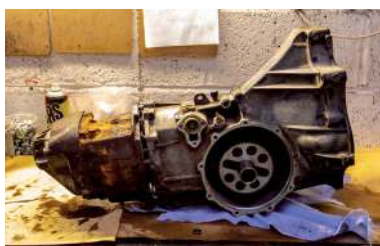
Far left Knackered bolts meant taking the gearbox casing apart required care and patience
