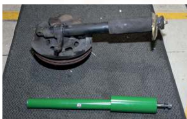
Above and right New Bilstein kit, complete with fresh front inserts for old Boge struts
